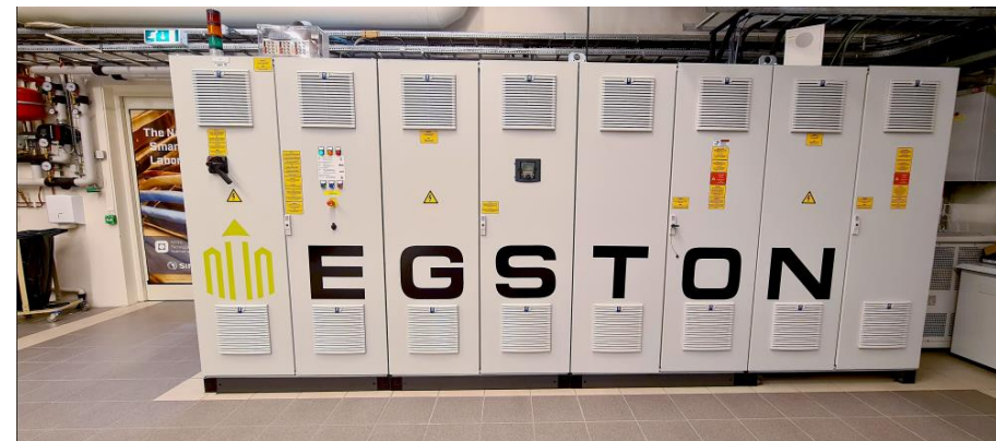
200 kVA controlled power amplifier with 5 kHz bandwidth
