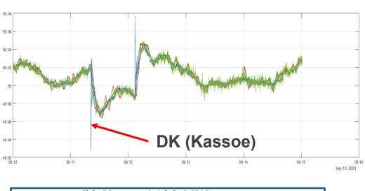
$$RoCoF = \frac{50 \, Hz}{8.1 \, s} \cdot \frac{1400 \, MW}{344000 \, MW} = 25, 1 \, mHz/s$$
